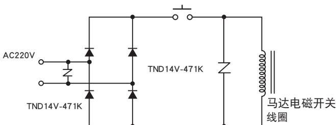
(6) 20kW马达控制回路 (Control of 20kW DC Motor)
