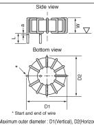
Maximum outer diameter : D1(Vertical), D2(Horizontal) Maximum width : W Total lead length \*1 : L=15±3mm
