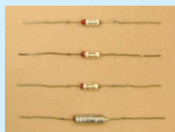
A micro electrolytic capacitor installed in the first model of transistor radio (produced in 1955)
