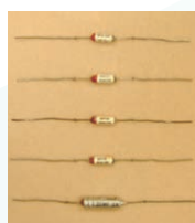
A micro electrolytic capacitor installed in the first model of transistor radio (produced in 1955)
