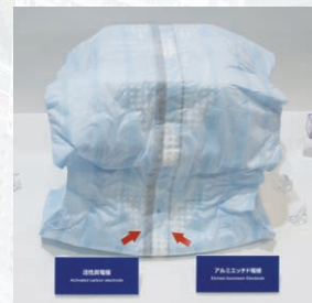
The two vertical lines are electrodes embedded inside the paper diaper. The right side is an aluminum etched foil and the left side is active carbon. To alleviate discomfort when wearing, the electrodes are made extremely thin and flexible.
