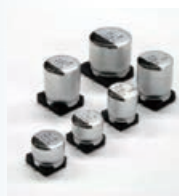
Conductive polymer hybrid aluminum electrolytic capacitors launched (2012)
