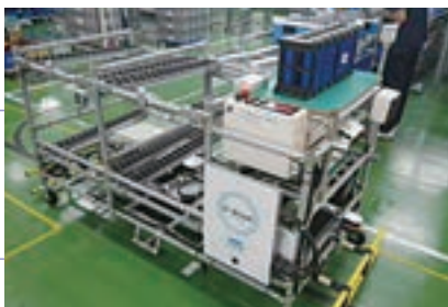
A capacitor-based wirelessly charged AGV in operation at Chemi-Con Nagaoka Corp., part of the Nippon Chemi-Con Group. The white plate on the side is a power receiver coil unit for wireless charging. This cart is used to transport components autonomously to the production line.
