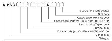
(Note2) PSC series,  $2.5V820\mu F(ESR 5m\Omega max.)$ has supplement code "J". Can case, terminal and terminal plating are the same as all others in PSC series.
