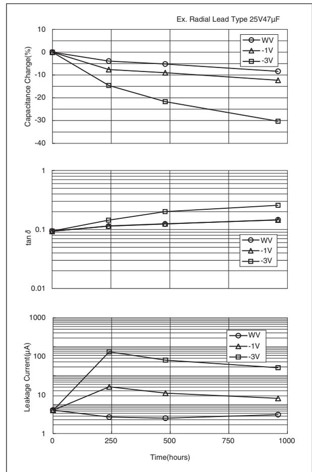
Fig-27 Applied Reverse voltage characteristic at 105°C
