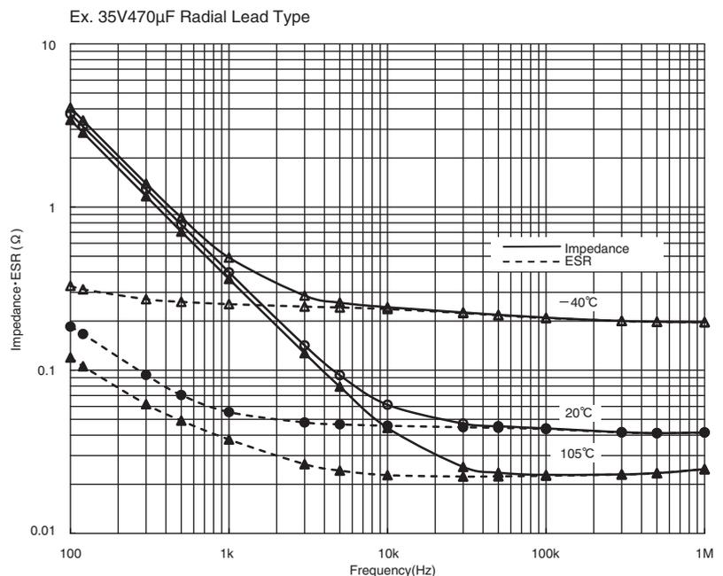
Fig-16 Temperature and Frequency Characteristics of Impedance · ESR
