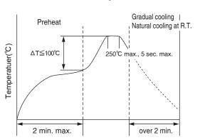
\*Flow Soldering Tin plating
